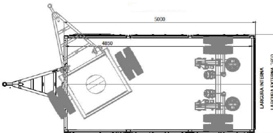
**Figura 6** - Vista superior semirreboque
